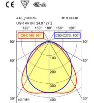
light source LED work equipment electronic ballast connected load 220-240 V, 50-60 Hz env. 55 W power consumption lens W optics, wide beam luminous flux approx. 8.300 lm luminous efficiency approx. 151 lm/W light type/-color cold white colour temperatur approx. 5.000 K color rendering index CRI > 80 light distribution direct direct ratio approx. 100 %
